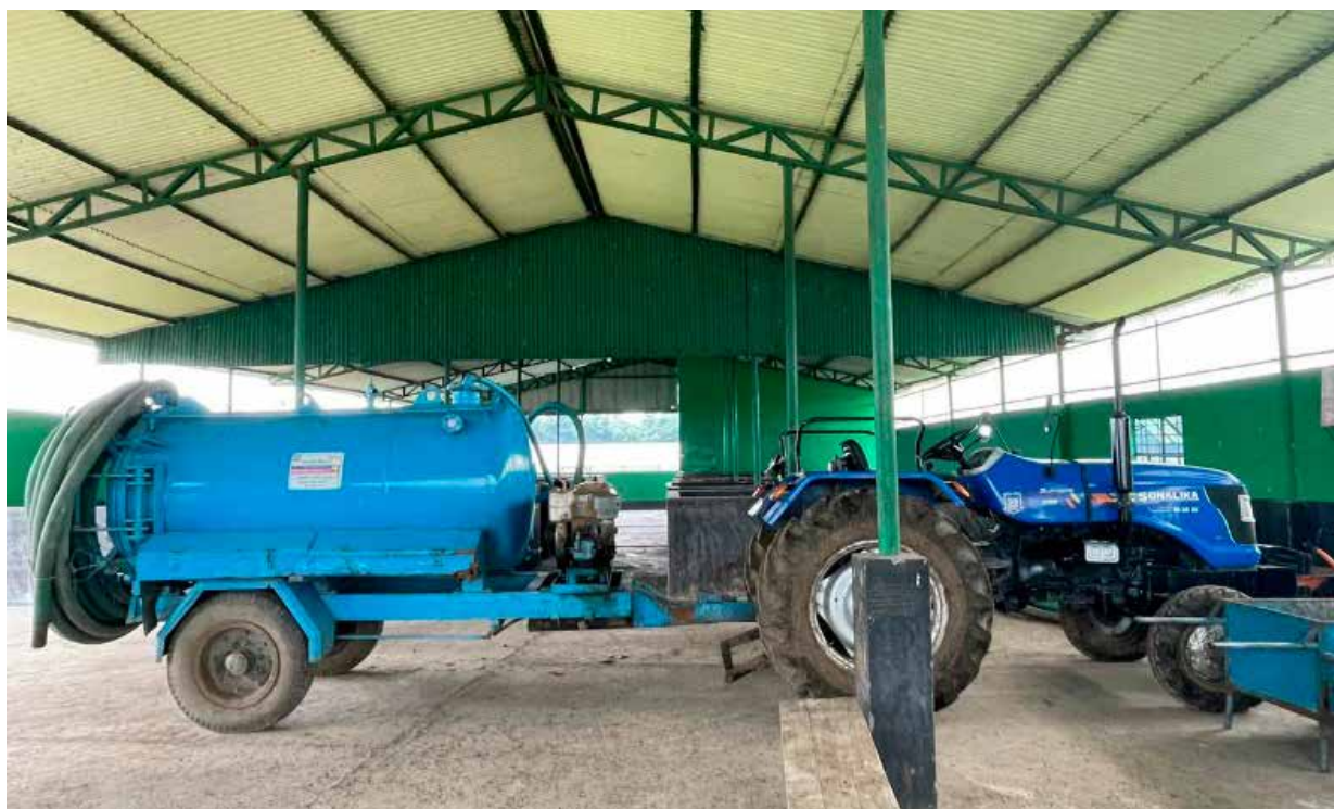
2000 litres capacity vacuum truck for collecting faecal sludge
